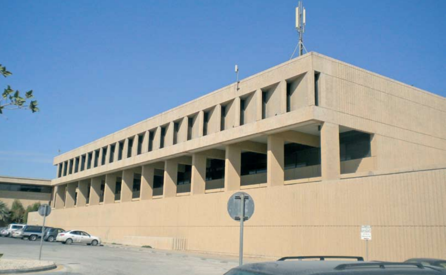
Fig. 2: Brise soleil – shading devices integrated with the building facade
