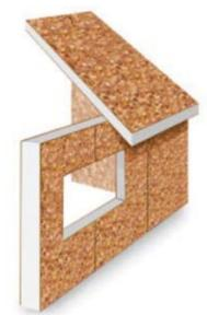
between two sheets of oriented strand board (OSB). You can consider SIPS green because of their superior insulation and air-sealing qualities, but they often must be set in place with a crane. SIPS construction is typically slightly more expensive than conventionally built structures.
